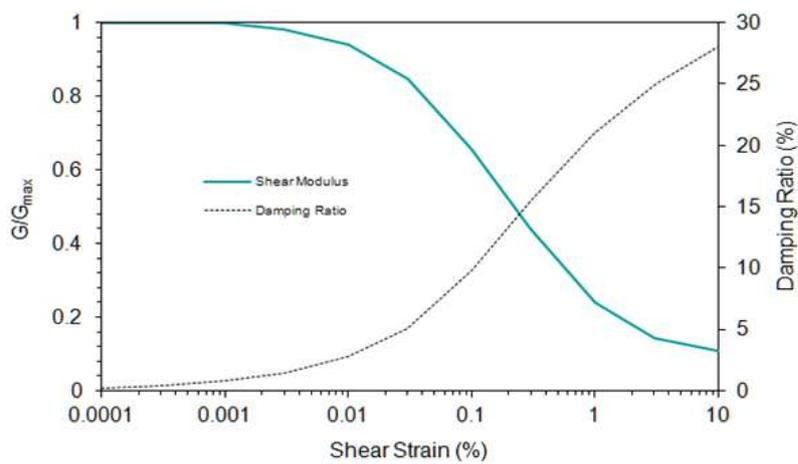
*Modulus for sand (Seed & Idriss 1970) - Upper Range and damping for sand (Idriss 1990) - (about LRng from SI 1970)*
